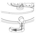
6. Refit the sump to the housing head by engaging the pins in the slots and turning the sump to the right until it is fully en-gaged.
