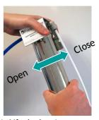
4. Lift the housing assembly off the retaining screws and holding the head firmly with one hand carefully unscrew the filter sump until it is free from the head. Empty the water from the filter sump and put the sump to one side.
