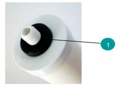
6. Check the new cartridge and the sealing washer (1) is correctly positioned. Check that the 'O' Seal inset in the top of the head (2) is correctly positioned. Screw the cartridge into the head until you feel the resistance of the washer meeting the sealing face. Continue to screw the cartridge a further ¼ turn to make an effective seal. Important note. Do not be tempted to over tighten the cartridge; over tightening will distort the sealing ring.
