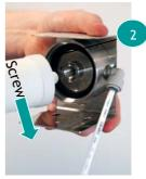
7. Tighten the sump firmly to make a watertight seal. Turn on the water supply and check the system for leaks. Leave the tap in the on position and allow the water to continue running for a minimum of 5 minutes to flush the cartridge. If the flow rate through the tap exceeds 2 lpm then adjust the shutoff valve flow rate down to 2 lpm. Your filter system is now fully operational and ready for use.
