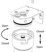
Install the filter cartridge and assemble the filter housing. Unscrew the housing to separate the head (E) from the sump (H). Holding the head in one hand screw the filter cartridge carefully in place, being careful not to over tighten it (see section 8 cartridge change instructions). Reassemble the housing to the sump and hand tighten it firmly.
