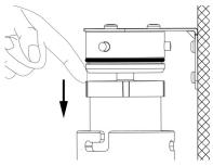
4. If the filter cartridge does not come away with the sump release it with an index finger by pushing down on the plastic rim.
